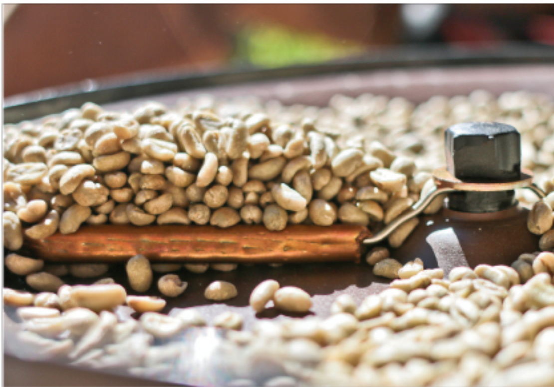
During the roasting process, green beans must stay in motion to avoid burning.
